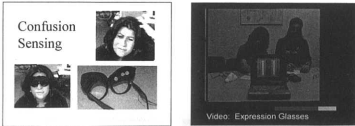
Figure 7. Expression glasses sense facial muscle changes and detect furrowing of the brow, a signal sometimes used to communicate confusion.
